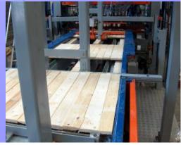
The machine concept allows also the maximum of automation due to the depots that accomplish the feeding of the transversal and longitudinal material. Under special requirements, the simultaneous nailing of block pallets is also possible.
